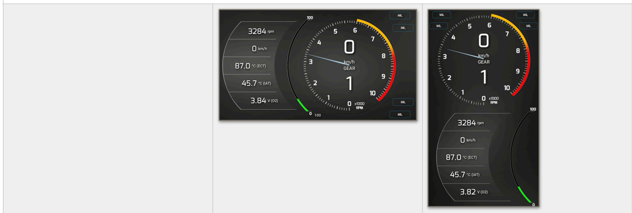
1 large analog style gauge with speed and gear (Gear display only available on specific protocol) and 5 digital gauge and 4 LED (LED's only available on specific protocol)
